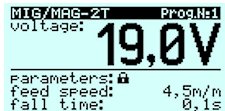
Welding arc source unit display in the MIG/MAG method
