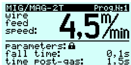
Wire feeder unit display in the MIG/MAG method
