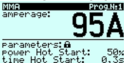
Welding arc source unit display during MMA welding
